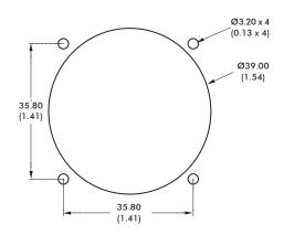
The joystick is dropped into the panel cut-out. For panel thickness of <3mm, M3 x 16 countersunk machine screws are recommended.
