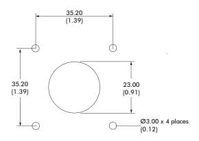
The body of the joystick is mounted from beneath the panel. The boot is passed through the panel cut-out and is held onto the front face of the panel by the mounting bezel. The square bezel has a gloss finish and is designed for use with No.4 x  $3/8^{\prime\prime}$  pan head self tapping screws whereas the circular bezel has a matt finish and is designed for countersunk screws.
