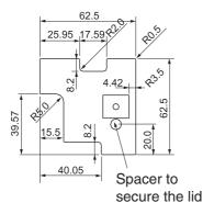
Enclosure for wall mounting. Suitable for sensors etc. Possiblity for 2 PCB's. PCB and packing are available. Standard colour is white/white but other colours can be supplied upon request.
