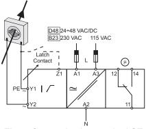
Fig. 4 Connection by standard CT
