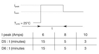
Note: Even though the D3 can withstand a slight increase in current for a limited time, it is not recommended for this purpose.
