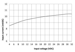
Fig. 3 RKD2 input current vs. input voltage
