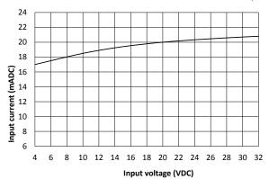
Fig. 4 RK2 input current vs. input voltage
