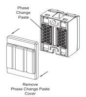
**Fig. 7** Remove cover before mounting on the panel chassis or heatsink.
