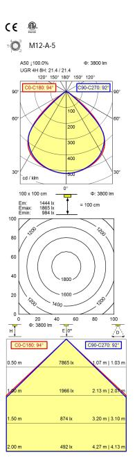
light source LED work equipment without connected load 24 V, DC env. 28 W power consumption luminous flux approx. 3.800 lm luminous efficiency approx. 136 lm/W light distribution direct 92° beam angle colour temperature neutral white colour temperatur approx. 5.000 K color rendering index (CRI) >= 80
