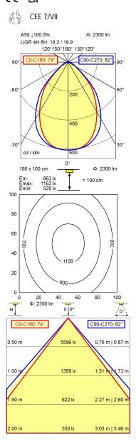
Light sourceLEDWork equipmentElectronic ballast dimable digitalConnected load220 - 240 V; AC; 50 Hz; 60 HzPower consumptionca. 32 WLuminous fluxapprox. 2.300 lm
