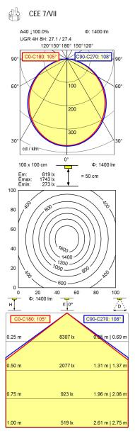
light source LED work equipment electronic transformer connected load 100 - 240 V; AC; 50 Hz; 60 Hz 24 V secondary tension power consumption ca. 23 W sec. power consumption ca. 19 W luminous flux approx. 1.400 lm
