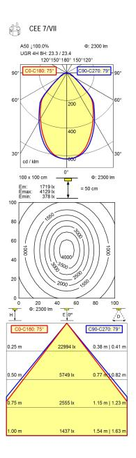
light source LED work equipment electronic transformer connected load 100-240 V, 50/60 Hz; secondary 24 V, DC power consumption env. 30 W luminous flux approx. 2.300 lm luminous efficiency approx. 88 lm/W light type/-color cold white colour temperatur approx. 4.000 K color rendering index CRI > 90; R9 > 50 light distribution direct direct ratio approx. 100 % beam angle 75°
