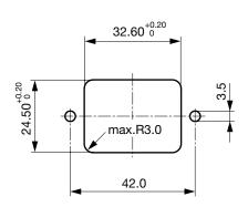
A = 32.0 mm; quick-connect terminals 6.3 x 0.8 mm A = 30.4 mm; quick-connect terminals 4.8 x 0.8 mm
